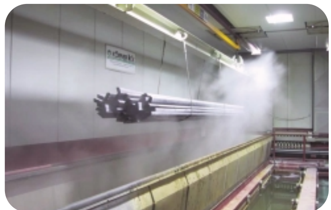
▲ Picture 3: Vapours from hot chemicals increase the relative humidity of the air
